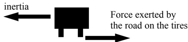
Here again we see the direction of inertia, and the opposite-acting force on the tires. But now we see that the force on the tires is acting where the tires meet the road, underneath the vehicle, but the inertia acts on the whole body of the vehicle—bottom, middle, and top.
